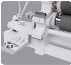
瓦楞輪探側吸設計 Corrugated Rolls Side Suction Design
