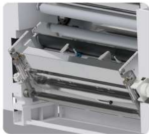
糊輪座可旋轉退出 Glue Unit By Rotation Way Eject
