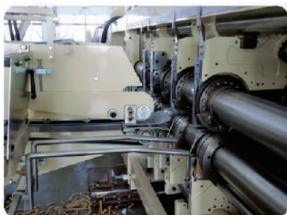
▼ 壓線/開槽部(雙開槽刀) Creasing / Slotting Unit (Dual Slotting Knife)
