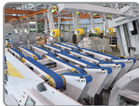
擋紙輪裝置(防止翻轉直接掉落) Sheet Sustain Unit (Rubber Stopper Wheels)
