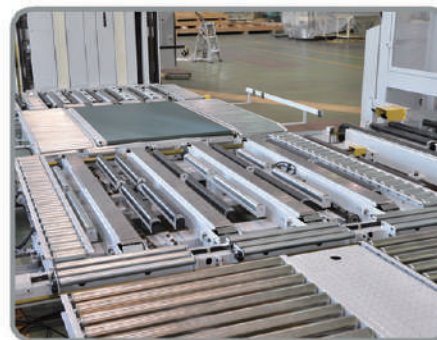
棧板與紙板的分離裝置 Push Out Pile Sheet from Pallet Device
